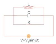
$$I = I_L + I_C + I_R = \frac{\phi}{L} + \frac{d}{dt}C\left(\frac{d\phi}{dt}\right) + \frac{1}{R}\frac{d\phi}{dt}$$
