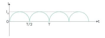
$$I_{rms}^{2} = \frac{\left\{ \left(I_{rms}\right)_{0-\frac{T}{2}}^{2} \right\} \frac{T}{2} + \left\{ \left(I_{rms}\right)_{\frac{T}{2}-T}^{2} \right\} \frac{T}{2}}{\frac{T}{2} + \frac{T}{2}}$$
