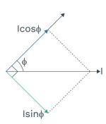
Hence Icos ∮ is the activity component of current because it is in phase with applied voltage. But Isin \( \phi \) is the component, which is inactive, called as wattless current because it is in  $\frac{\pi}{2}$ phase with applied voltage.
