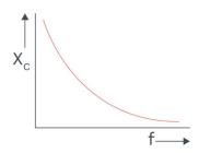
Capacitive reactance  ${\rm 'X_{\rm c}'}$  is inversely proportional to frequency of A.C.
