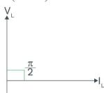
In a pure inductive circuit current always lags behind the emf by  $\frac{\pi}{2}$  or alternating emf leads the
