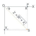
The term  $(R^2 + X_c^2)$  represents the effective resistance of the R-C circuit and called the capacitive impedance  $Z_{\rm c}$  of the circuit.
