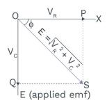
The vector OP represents  $\rm V_{\rm R}$  (which is in phase with I) and the vector OQ represents  $\rm V_{\rm C}$  (which
