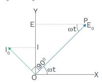
In a pure capacitive circuit, the current always leads the e.m.f. by a phase angle of  $\frac{\pi}{2}$ . The alternating emf lags behind the alternating current by a phase angle of  $\frac{\pi}{2}$ .
