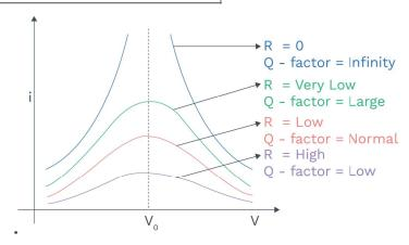
According to figure, if 'R' is decreasing means Q-factor or sharpness will increase in the circuit.
