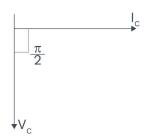
Let at any instant t charge on the capacitor = q Instantaneous potential difference across the capacitor E = q/C
