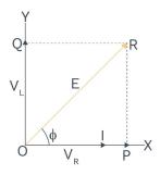
Then  $V_L = IX_L$  and  $V_R = IR$ Now,  $V_R$  is in phase with the current while  $V_L$  leads the current by  $\frac{\pi}{2}$ .
