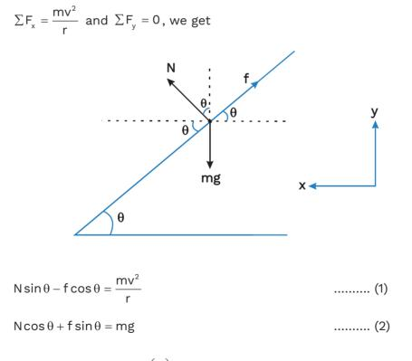
Substituting,  $\theta = \tan^{-1}\left(\frac{1}{2}\right)$ ,  $v = 5 \text{ ms}^{-1}$ , m = 200 kg and r = 20 m, in equation (1) and (2), we get  $f = 300\sqrt{5} \text{ N}$  (outwards)
