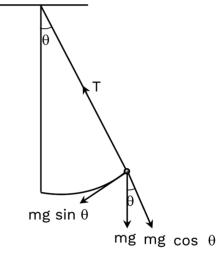
(b) Since  $a_c$  is provided by  $(T - mg \cos \theta)$  acting radially inwards, so  $a_c = \frac{T - mg \cos \theta}{r} = \frac{v^2}{r}$ .
