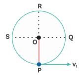
The particle is in equilibrium. Let the particle be given an initial velocity  $\overline{v}_1$  in horizontal direction as, shown in figure. The particle moves along a vertical circle (radius = length of the string). The point of suspension is the centre of the circle.
