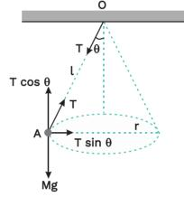
Let T be the tension in the string of length l and r be the radius of circular path. The vertical component of tension T balances the weight of the bob and horizontal component provides the necessary centripetal force. Thus,
