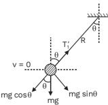
Now, when the ball reaches its bottom-most point, it has acquired a velocity v. At this point, T-mg =  $ma_c$
