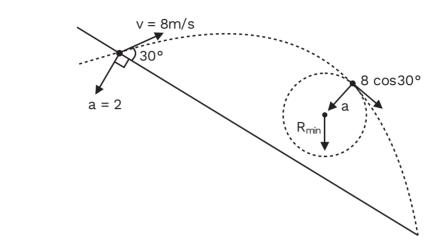
Radius of curvature will be minimum at the point where speed is minimum.
