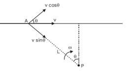
A man is standing 3m from a wall and he lights up a torch on the wall. If he is rotating the torch at an angular speed of 0.1 rad/s, then what is the velocity of spot of light when light ray makes an angle of 45° with the line joining the man and wall.
