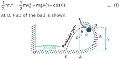
As the ball leaves the track at D, normal reaction is zero. By Newton's 2<sup>nd</sup> law in radial direction,
