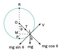
To get the basic characteristics of vertical circular motion, consider an instantaneous position of the particle at point L.
