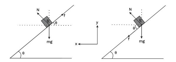
The direction of second force, i.e., normal reaction N is also fixed (perpendicular to road).
