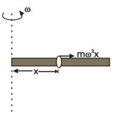
Velocity at time of leaving the rod is the resultant of tangential speed and the radial speed of the particle. So,
